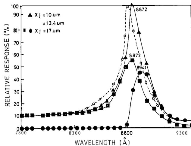
FIG. 7 Experimental spectral response of fabricated photodiodes. Note that sample of  $x_j = 10 \mu\text{m}$  is in good agreement to the prediction (blank circle) of Fig. 4.
