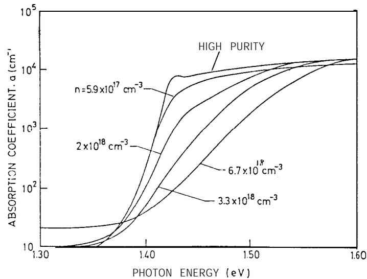
FIG. 2 The variation of absorption coefficient with respect to wavelength and the concentration in n-type GaAs. (from ref. 2,3,4)
