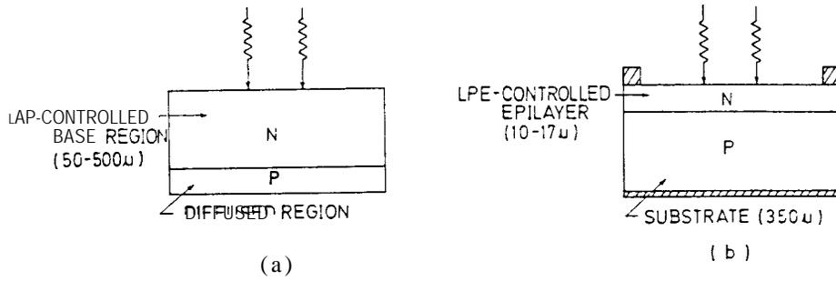
FIG. 1 The structures of narrow-band self-filtering photodiodes. a) M.B. Prince's method' with back-illumination, base region is lapped to a proper thickness; b) Our LPE method with front-illumination
