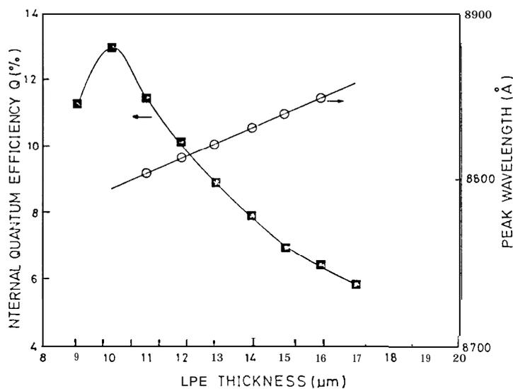
FIG. 5 Theoretical calculation of the thickness effect on the peak wavelength and the internal quantum efficiency.
