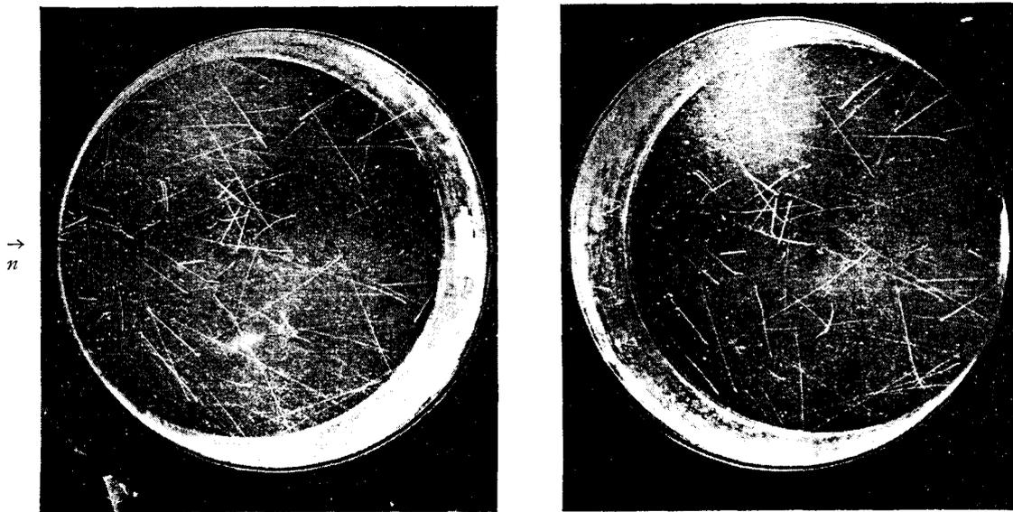
Fig. 2. An example of the stereoscopic picture of disintegrations produced by 11.1 Mev neutrons. The arrow indicates their direction of incidence. The chamber is filled with 1 atmos. argon-gas and water mixture. ( $f=16$ , Kodak Plus-X Pan).
