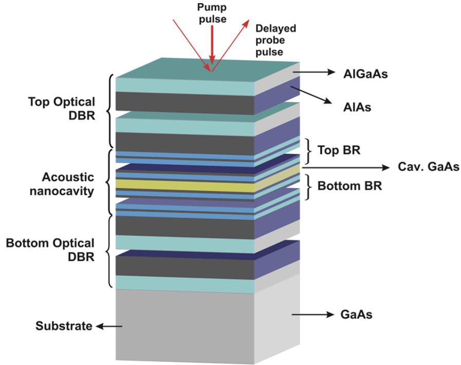
FIG. 1: Schematics of the sample and the experimental geometric configuration. Two optical DBRs are separated by an optical spacer constituted by an acoustic nanocavity. The pump and probe pulses impinge from the top side of the sample.
