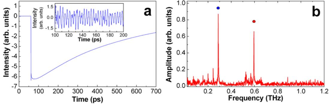
FIG. 2: Coherent phonon generation experiments. Panel a: time resolved reflectivity measured in an optical microcavity with the laser tuned with the optical mode. Inset: detail of the derivative of the signal between 100 and 200 ps after the application of a bandpass filter (200–900 GHz). Panel b: Fourier transformation of the time trace shown in panel a. Peaks indicated with circles correspond to confined acoustic cavity modes (see text for details).
