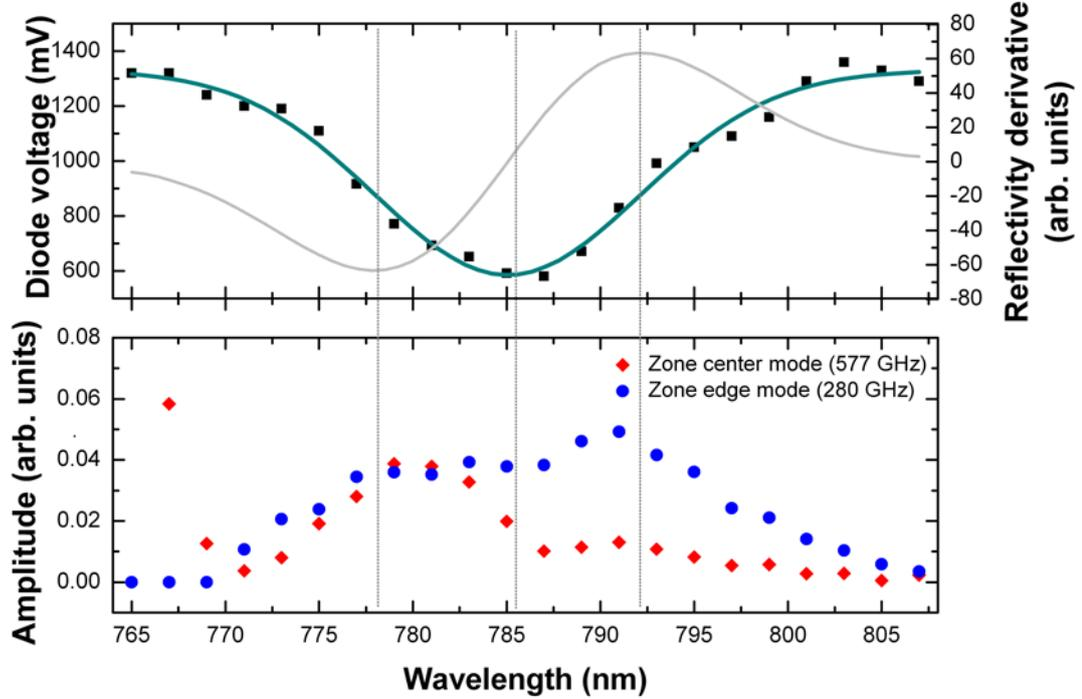
FIG. 3: Coherent phonon generation in an optical microcavity. Top panel: Optical reflectivity measured as a function of the laser wavelength (squares). The green line is a gaussian fit. In gray, the derivative of the fitting curve. Bottom panel: intensity of the cavity modes as a function of the laser wavelength. Blue (red) dots correspond to the zone edge (center) cavity mode. Vertical lines indicate the cavity mode wavelength (central line) and maximum and minimum derivative.
