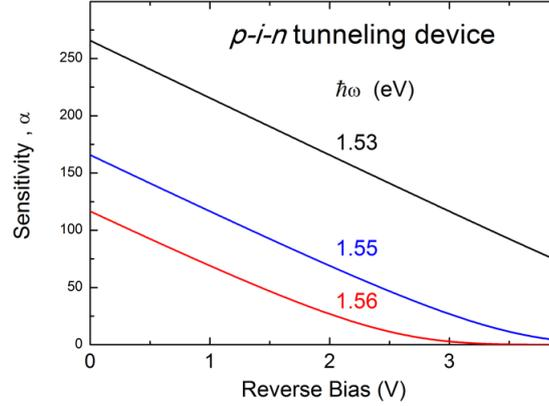
FIG. 7: Calculated dependency of the photocurrent sensitivity  $\alpha$  to the strain for three excitation-photon energies. The calculations are performed for the p-i-n structure used in the experiments.
