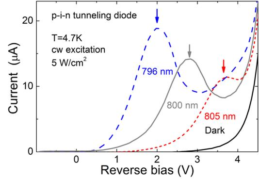
FIG. 2:  $I$ - $V$  curves measured in the dark and under illumination for different wavelengths of CW optical excitation.
