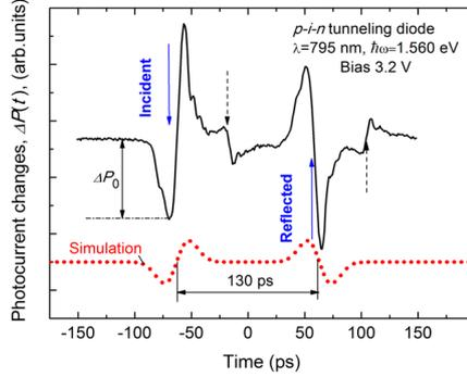
FIG. 5: The temporal trace (solid line) of the photocurrent changes. Solid vertical arrows indicate the arrival of the middle of incident and reflected strain pulses. Dashed vertical arrows show the next echoes generated in an Al film transducer. The dotted line is the simulated temporal trace when the incident and reflected bipolar strain pulses pass through the QW.
