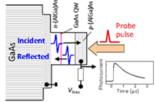
FIG. 4: The schematic diagram of ultrafast probing of the photocurrent changes in the p-i-n structure, showing the bipolar strain pulses arriving at the QW due to the initial strain pulse and the pulse reflected from the top surface of the device.
