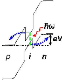
FIG. 1: The band diagram of p-i-n diode with a QW when the reverse bias is applied. The dashed vertical and curved lines show optical and tunneling transitions in the QW.
