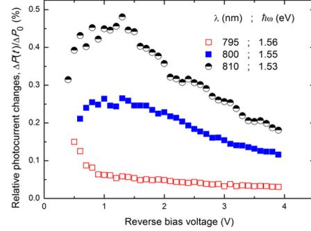
FIG. 6: The dependencies of the relative photocurrent changes amplitude  $\Delta P_0/P_0$  on reverse bias voltage measured for three various excitation wavelengths  $\lambda$ . Corresponding photon energies  $\hbar\omega$  are also indicated.
