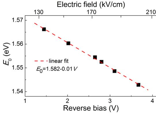
FIG. 3: Bias dependence of the exciton resonance energy  $E_0$  of the QW, obtained from the position of peaks in the  $I$ - $V$  curves for various excitation wavelengths. The upper horizontal scale shows the electric field in the QW calculated from the experimental values of  $E_0$ .
