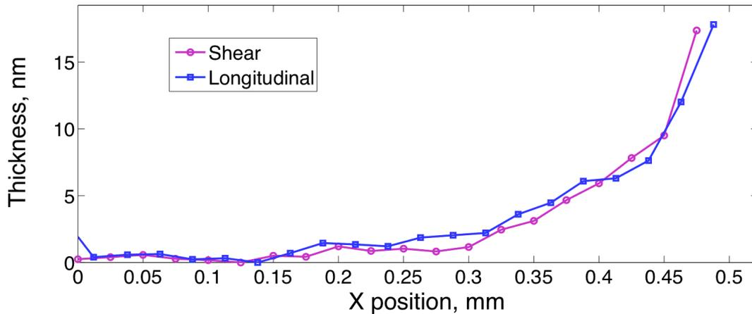
FIG. 5: Topography of a water layer at room temperature calculated from Brillouin scattering measurements at 42 GHz (longitudinal) and 25 GHz (shear).
