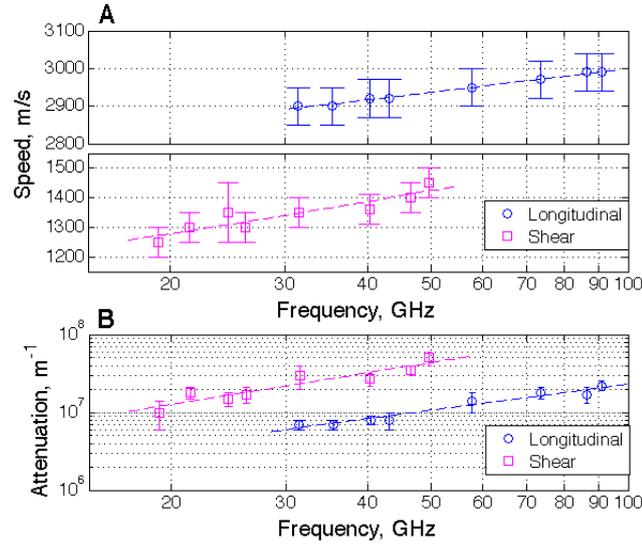
FIG. 4: Results of shear and longitudinal acoustic speeds (A) and attenuation coefficients (B) in liquid glycerol at room temperature.
