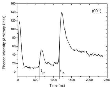
FIG. 2: Time trace of phonon intensity through 2.8 mm of  $\text{CaWO}_4$  at the (001) point in Fig. 1(a). The initial pulse is the direct excitation of the detector by scattered laser light. The times  $t_{\text{LA}} = 613$  ns and  $t_{\text{TA}} = 1170$  ns correspond to the arrival of the longitudinal and transverse acoustic waves along this direction.
