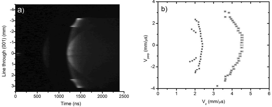
FIG. 3: (a) Position vs. time plot of phonon intensities along the center scan line shown in Fig. 1(a) ([001]-oriented sample). (b) Group velocities calculated from the arrival times shown in part (a).
