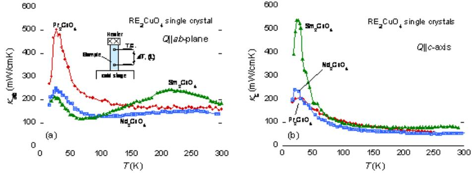
FIG. 1: Temperature dependence of the thermal conductivity (a) in the  $ab$ -plane and (b) along the  $c$ -axis,  $\kappa_{ab}(T)$  and  $\kappa_c(T)$ , respectively, of the Pr214, Nd214, and Sm214 single crystals.
