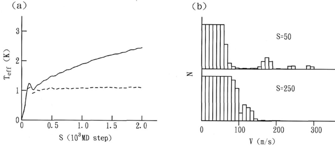
FIG. 5: Variation in the effective temperature in the crystal in which hot atoms are injected. The dashed line shows the result for a perfect crystal and the solid line is for a crystal with dislocation (a). Histograms of velocity distribution at typical time steps (b).
