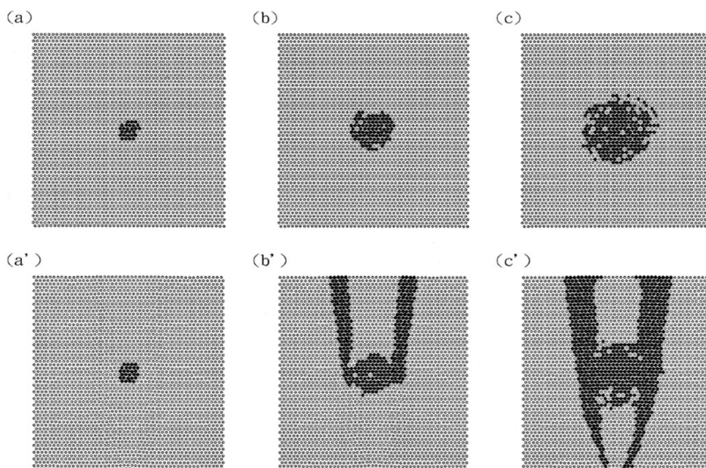
FIG. 4: Evolution of hot atoms at (a) 50 MD step, (b) 250 MD step, and (c) 750 MD step in a perfect crystal. Solid circles show hot atoms. Figures (a'), (b') and (c') show the evolution at same MD steps in a crystal with dislocation.
