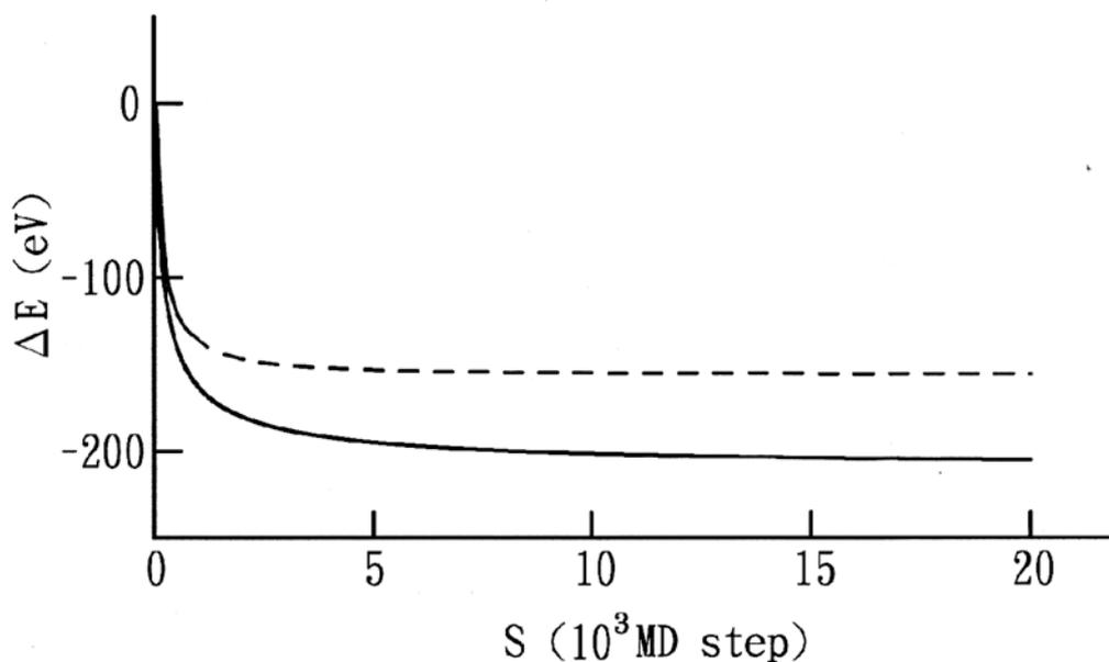
FIG. 3: Change in the total potential energy through initial relaxation. Solid line shows the result for fixed-boundary condition, and dashed line is for free-boundary condition.
