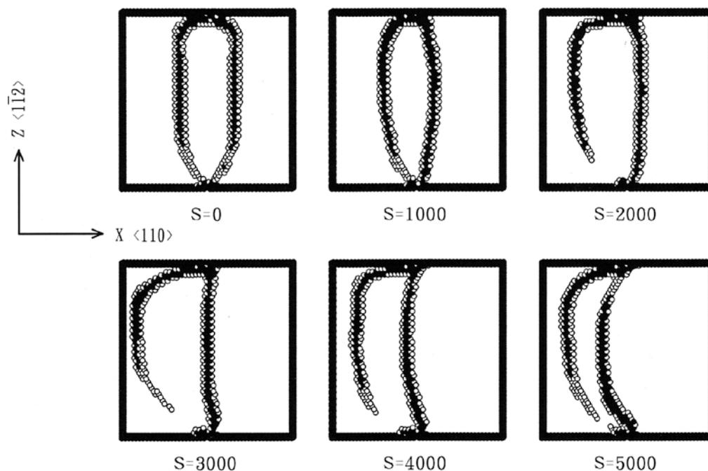
FIG. 6: Motion of split edge dislocation under a fixed-boundary condition.  $S$  represents MD time steps. The indication for atoms is the same as that in figure 1.
