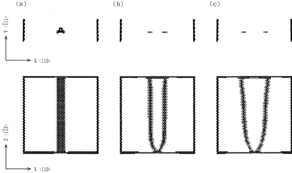
FIG. 2: Configuration of atoms around an edge dislocation (a) before, (b) in the middle of, and (c) after the initial relaxation under the free-boundary condition. The indication is the same as that of figure 1.
