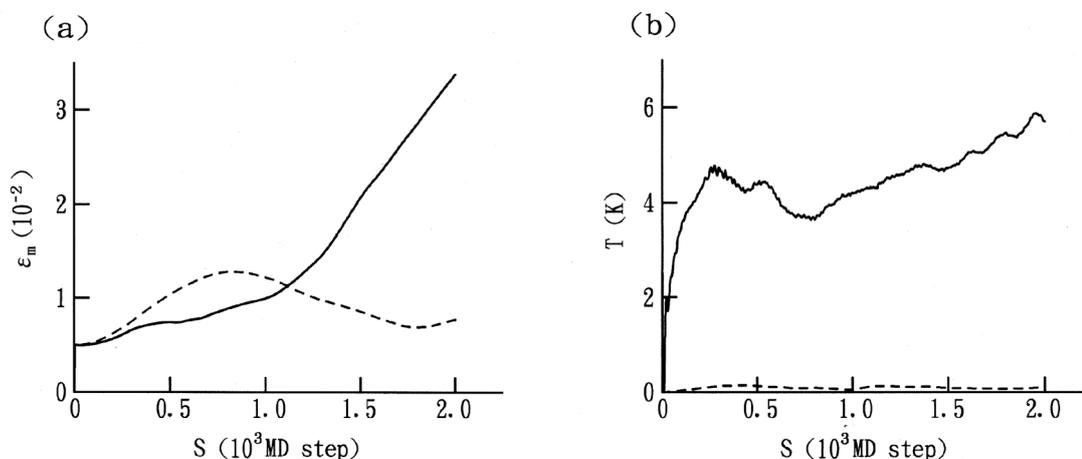
FIG. 8: (a) Change in mean strain  $\epsilon_m$  and (b) mean temperature  $\bar{T}$  in the crystal with moving dislocation. The solid lines show the results for the free-boundary condition and the dashed line shows the results for fixed boundary.
