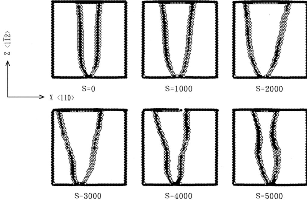
FIG. 7: Motion of split edge dislocation under a fixed-boundary condition.  $S$  represents MD time steps. The indication for atoms is the same as that in figure 1.
