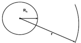
FIG. 1: Schematic of the studied sample geometry. A circular heater with radius  $R_h$  emits phonons, which can be detected by a thermometer of length  $l$  placed at a distance  $r$  from the center of the heater.
