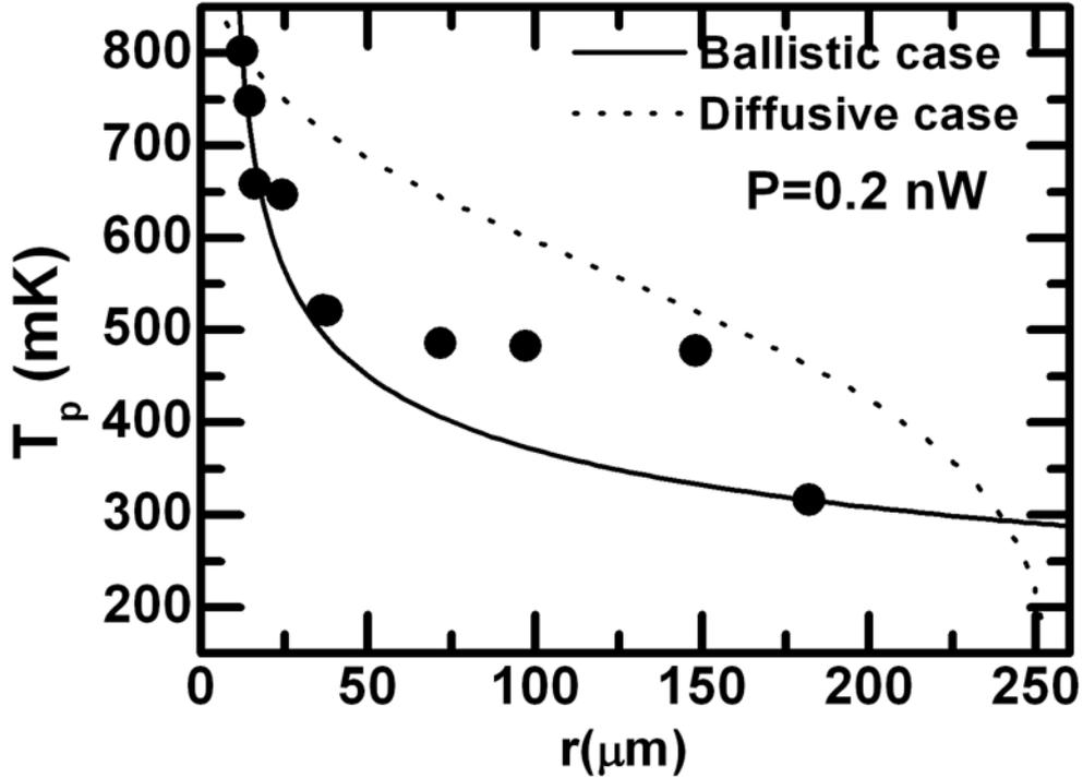
FIG. 3: Plot of local phonon temperature  $T_p$  versus distance from the center  $r$  at constant heating power  $P = 0.2\text{nW}$ . Black dots: measured data. Black solid line: data obtained for the ballistic model from Eq. (3). Black dotted line: data obtained for the diffusive model from Eq. (9).
