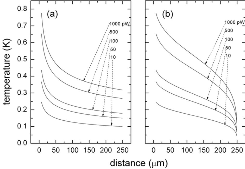
FIG. 2: Theoretical temperature profiles for (a) ballistic [Eq. (5)] and (b) diffusive [Eq. (9)] phonon transport in membranes for radially symmetric geometry. Different curves correspond to varying input powers in sequence  $P = 10, 50, 100, 500, 1000$  pW.
