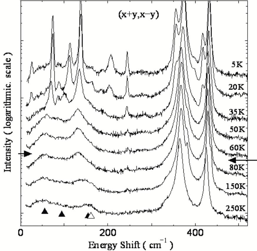
FIG. 2: Temperature dependence of Raman spectra of  $\text{PrRu}_4\text{P}_{12}$ . For details, see text.
