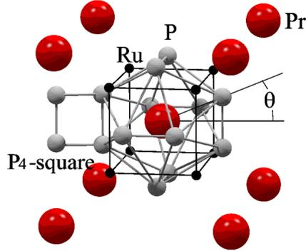
FIG. 1: Crystal structure of skutterudite compound  $\text{PrRu}_4\text{P}_{12}$ . The P and Ru ligands around the 8 Pr ions at the corner positions are not depicted. For more details, see text.
