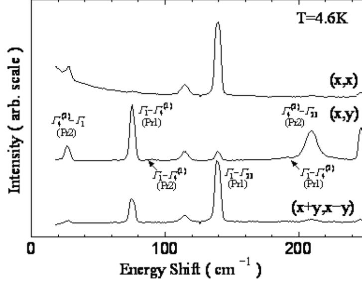
FIG. 4: Polarization dependence of Raman spectra of  $\text{PrRu}_4\text{P}_{12}$  at 4.6 K.
