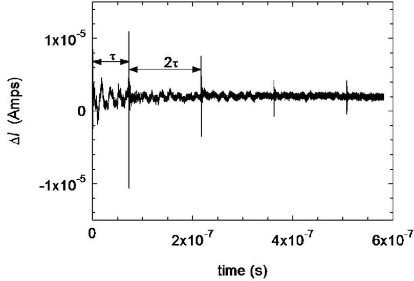
FIG. 2: Signal at an applied forward bias of 1V. The laser pulse is incident on the Al film at time  $t = 0$ . After time  $\tau \approx 72ns$ , the acoustic pulse reached the diode device. Multiple reflections of the acoustic pulse can be seen, which are separated in time by  $2\tau$ .
