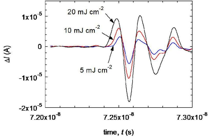
FIG. 4: Signal at 0 V bias for three different values of the excitation laser intensity.
