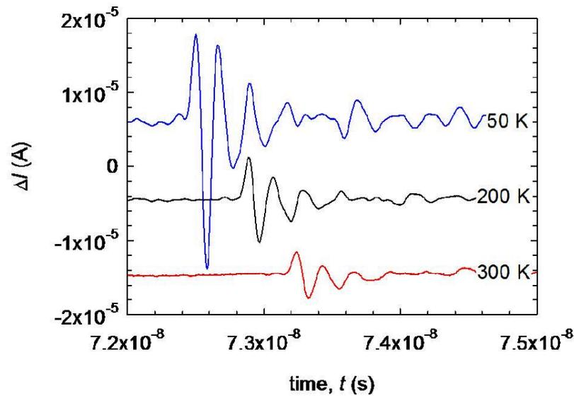
FIG. 5: Signals at 0 V bias for three different sample temperatures (traces are offset vertically for clarity).
