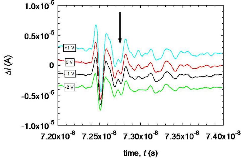
FIG. 3: Signal arriving at  $\tau \approx 72\text{ns}$  on a zoomed time axis, for four different values of the DC bias applied to the device (traces are offset for clarity). The arrow indicates the expected time of arrival back at the  $p$ - $n$  junction of the acoustic pulse reflected from the top of the device.
