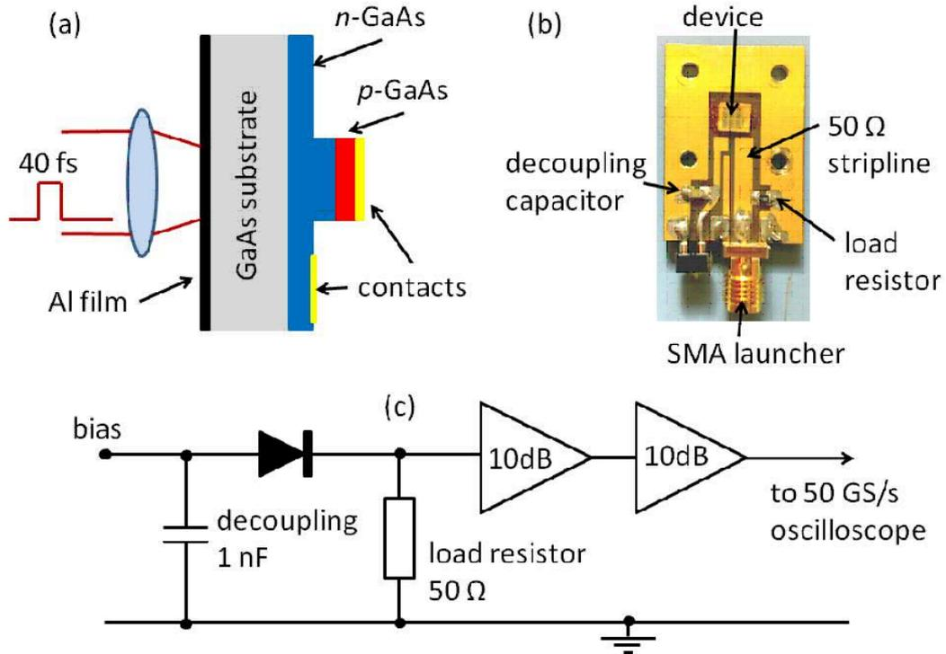
FIG. 1: Experimental arrangement: (a) sample schematic; (b) sample holder; (c) circuit diagram.
