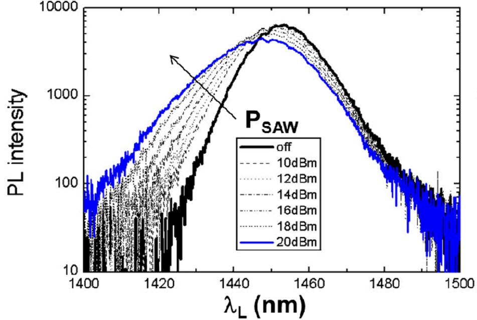
FIG. 2: Photoluminescence (PL) spectrum of the InGaAsP structures at 10 K. The PL measurements were carried out under confocal excitation and detection for different rf-power  $P_{SAW}$  applied to the acoustic transducer.
