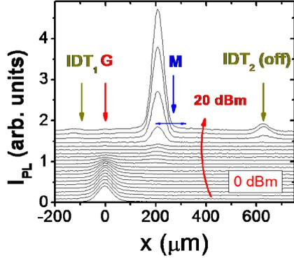
FIG. 4: Integrated PL profiles along the SAW transport path for different nominal rf-powers ( $P_{SAW}$ ) applied to IDT<sub>1</sub> (cf. Fig. 2(a)).  $P_{SAW}$  was varied in steps of 1 dBm from 0 (lowest curve) to 20 dBm (highest curve).
