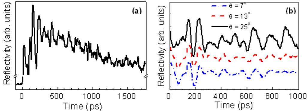
FIG. 2: (a) Temporal evolution of reflectivity induced by coherent elastic vibrations in the studied sample. Moment  $t = 0$  corresponds to the pump excitation. (b) Temporal evolution of reflectivity after subtraction of “step-like” background for different incident angles of the probe beam.
