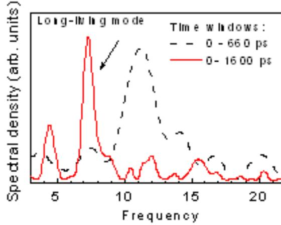
FIG. 3: Power spectral density obtained by FFT of the measured reflectivity  $\Delta R(t)$  as a function of vibration frequency. The solid and dashed curves represent the spectra obtained for long ( $\Delta t = 1600$  ps) and short ( $\Delta t = 660$  ps) time windows, respectively.
