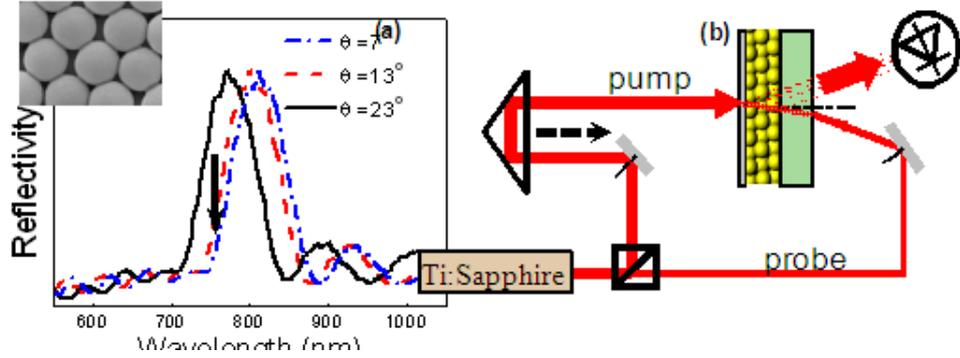
FIG. 1: (a) Reflectivity spectra of studied sample measured at different incident angles. Vertical arrow shows the wavelength of the probe laser. SEM image of top layer of that sample is presented in the inset. (b) Setup of the pump-probe experiments.
