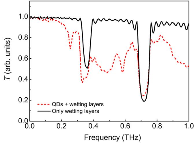
FIG. 4: Calculated amplitude transmission  $T$  spectra of the QD crystal, including QDs and wetting layers, and a similar structure without considering the QDs, i.e., only wetting layers.
