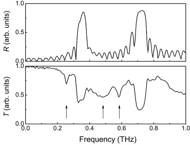
FIG. 3: Calculated amplitude reflection  $R$  (top) and transmission  $T$  (bottom) spectra of the QD crystal. The arrows denote the transmission reduction (250, 480, and 580 GHz) in addition to the effect of phononic band gaps.
