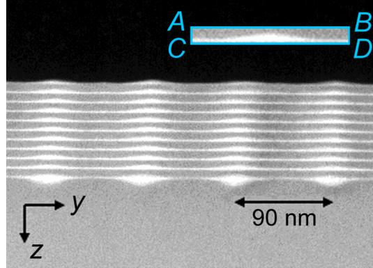
FIG. 1: TEM imaging of the studied QD crystal without the Si cap layer. The inset shows a unit cell of this nanocrystal.
