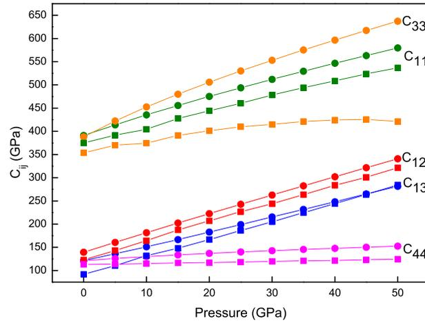
FIG. 1: A comparison for the elastic constants of w-AlN.
