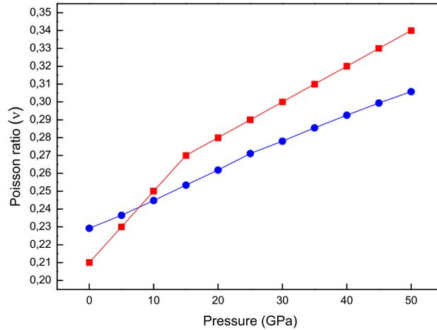
FIG. 3: Poisson ratio of w-AlN under pressure.
