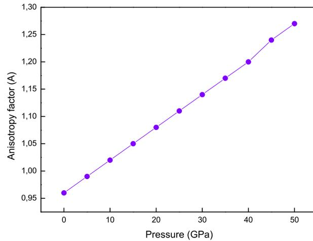
FIG. 6: Pressure dependency of the anisotropy factor for w-AlN.
