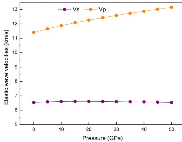
FIG. 4: Elastic wave velocities of w-AlN vs. pressure.
