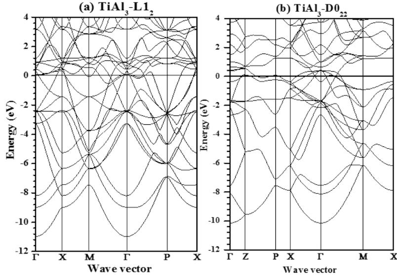
FIG. 2: Band structures along high-symmetry lines of the two phases (a)  $L1_2$  and (b)  $D0_{22}$  in  $\text{TiAl}_3$  intermetallic alloy system. The solid horizontal line represents the Fermi level ( $E_F = 0$  eV).
