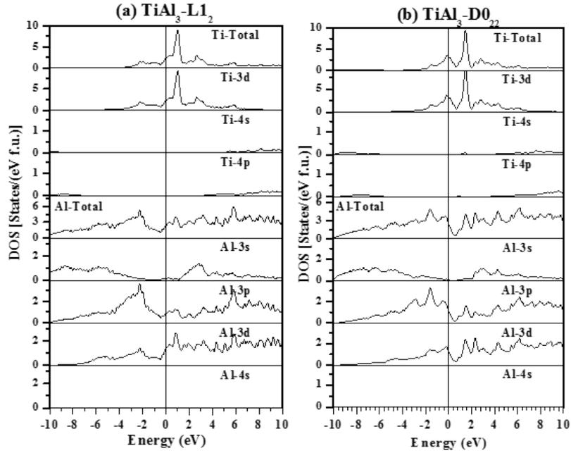
FIG. 4: Total and orbital resolved partial DOS plots of the two phases (a)  $L1_2$  and (b)  $D0_{22}$  in  $TiAl_3$  intermetallic alloy system.
