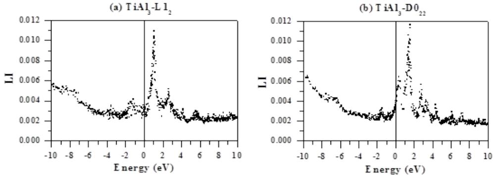
FIG. 5: Localization index (LI) plots of the states of the two phases (a) L1<sub>2</sub> and (b) D0<sub>22</sub> of TiAl<sub>3</sub> intermetallic alloy system.
