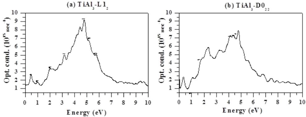
FIG. 7: Optical conductivity spectra of the two phases (a)  $L1_2$  and (b)  $D0_{22}$  of  $TiAl_3$  intermetallic alloy system.
