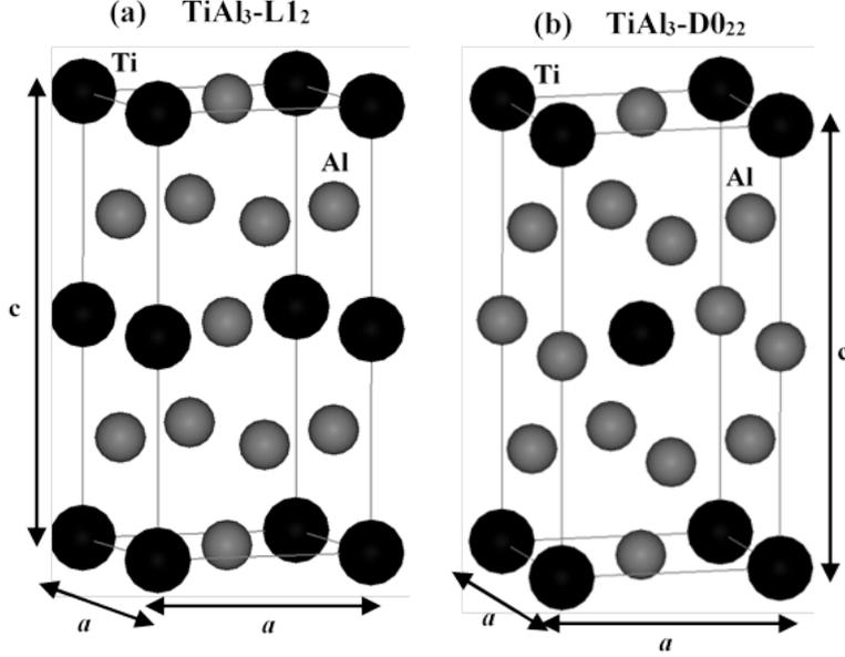
FIG. 1: Crystal structures of the two phases (a) L1<sub>2</sub> and (b) D0<sub>22</sub> in TiAl<sub>3</sub> intermetallic alloy system. Dark black circles represent Ti atoms, while grey circles stand for Al atoms.
