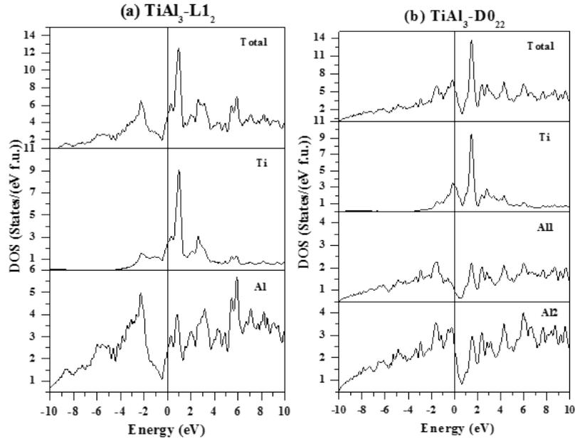
FIG. 3: Total and element resolved partial DOS plots of the two phases (a)  $L1_2$  and (b)  $D0_{22}$  in  $TiAl_3$  intermetallic alloy system.
