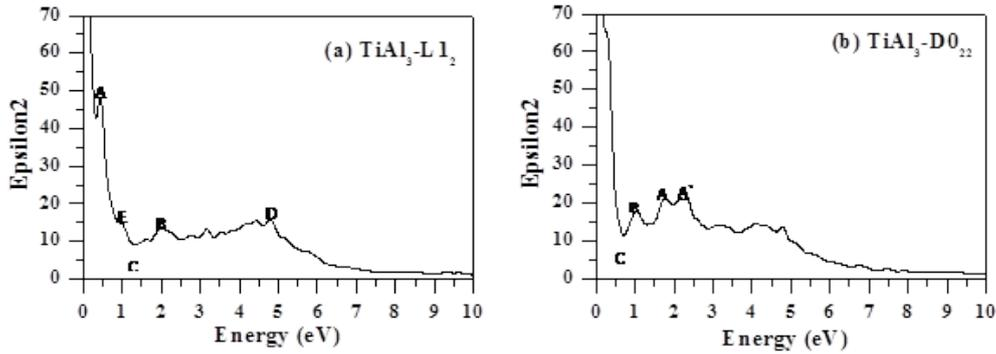
FIG. 6: Calculated imaginary part of the dielectric function of the two phases (a)  $L1_2$  and (b)  $D0_{22}$  of  $TiAl_3$  intermetallic alloy system.
